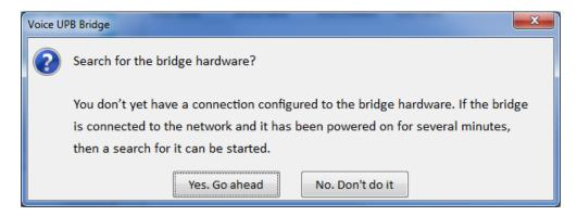
You should attempt the finds operation. The Bridge must be powered on for several minutes before it is working and capable of being found by the Bridge software. If the find operation is successful, then the IP address of the Bridge displays.
